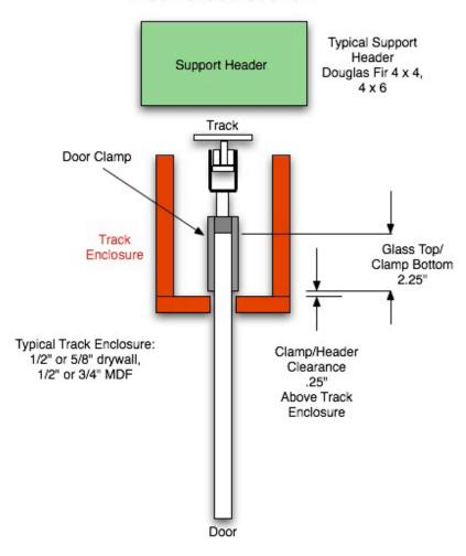
The glass clamp will cover the top side of the glass by 2.25" from the top of the door down to the bottom edge of the clamp side wall.
