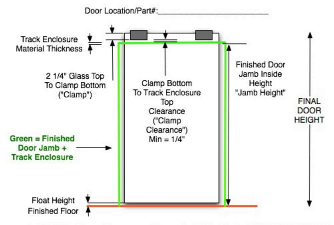
Jamb Height + Clamp Clearance + Clamp + JambMat - Float = FINAL DOOR HEIGHT (Typical: (80"H + .25" Clear + 2.25" Clamp + .5" Enclosure) - Float .25" = Final 82.500")
