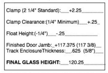
The factors related to calculating the glass door height based on a desired finished height are:
